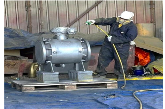
SPRAY PAINTING – FLOWSERVE VALVES
